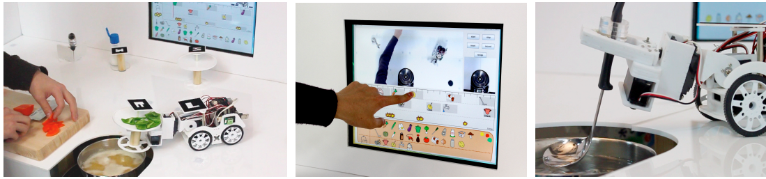
Figure 1: Left: Overview of the system. Center: Graphical user interface. Right: Robot stirs the pot.
